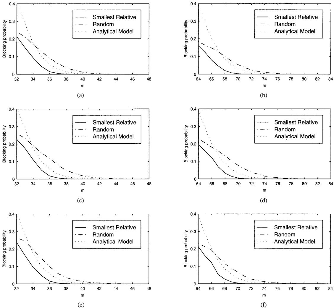
Fig. 8. The comparison between the analytical model and the simulation results for the  $v(m, 32, 32)$  and  $v(m, 64, 64)$  multicast networks. (a)  $N = 1024$  under uniform traffic. (b)  $N = 4096$  under uniform traffic. (c)  $N = 1024$  under uniform/constant traffic. (d)  $N = 4096$  under uniform/constant traffic. (e)  $N = 1024$  under Poisson traffic. (f)  $N = 4096$  under Poisson traffic.
