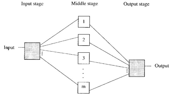
Fig. 2. The paths between a given input and output pair in the  $v(m, n, r)$  network.
