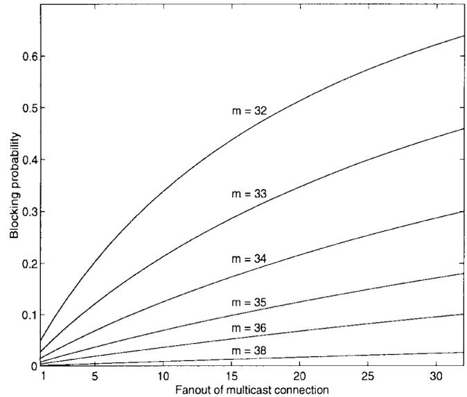
Fig. 5. Blocking probabilities for  $v(m, 32, 32)$  network with fanouts between 1 and 32.  $N = 1024$ ,  $n = r = 32$ , and  $a = 0.7$ .
