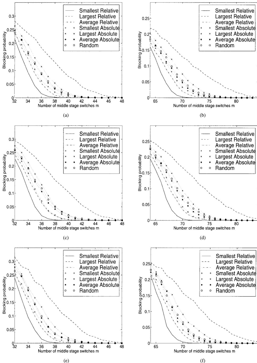
Fig. 6. The blocking probability of the  $v(m, 32, 32)$  and  $v(m, 64, 64)$  multicast networks under seven routing control strategies. (a)  $N = 1024$  under uniform traffic. (b)  $N = 4096$  under uniform traffic. (c)  $N = 1024$  under uniform/constant traffic. (d)  $N = 4096$  under uniform/constant traffic. (e)  $N = 1024$  under Poisson traffic. (f)  $N = 4096$  under Poisson traffic.
