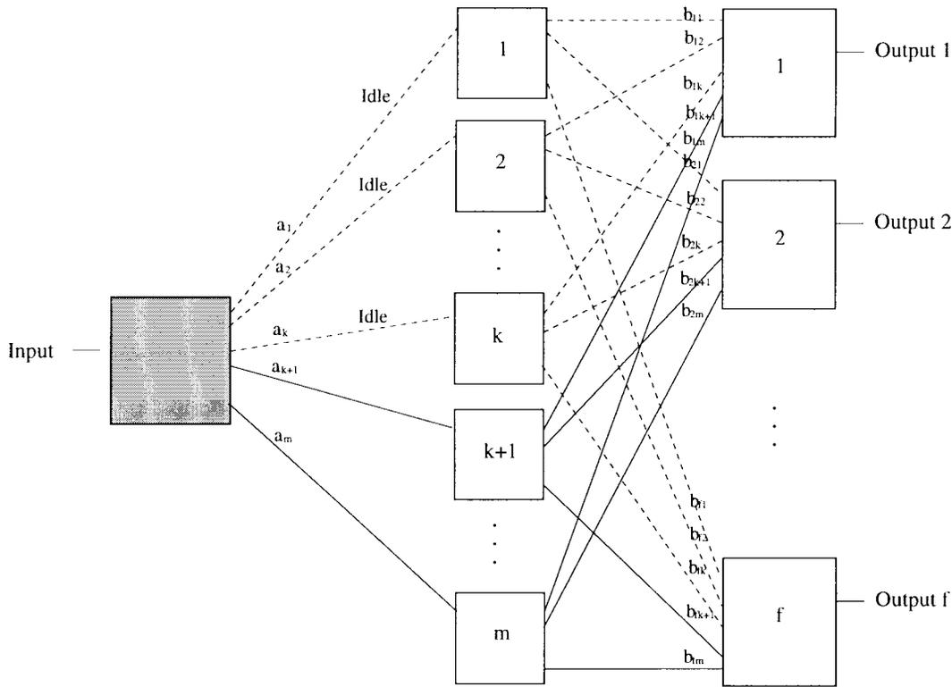
Fig. 3. The subnetwork associated with a multicast connection with fanout  $f$ . The dashed lines indicate the idle link subnetwork.
