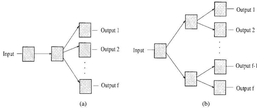
Fig. 4. Different ways to realize a multicast connection. (a) Fanout to one middle switch. (b) Fanout to two middle switches.
