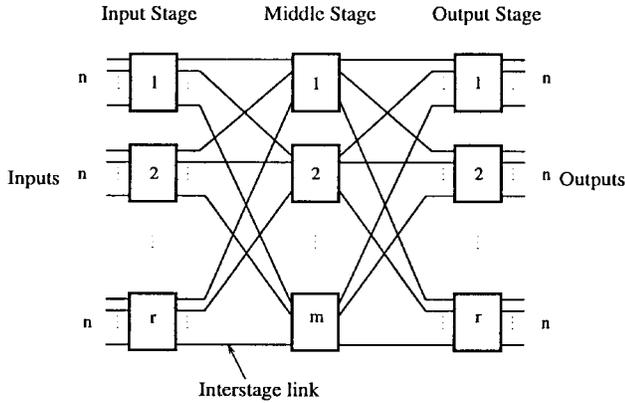
Fig. 1. A general schematic of an  $N \times N$   $v(m, n, r)$  network, where  $N = nr$ .
