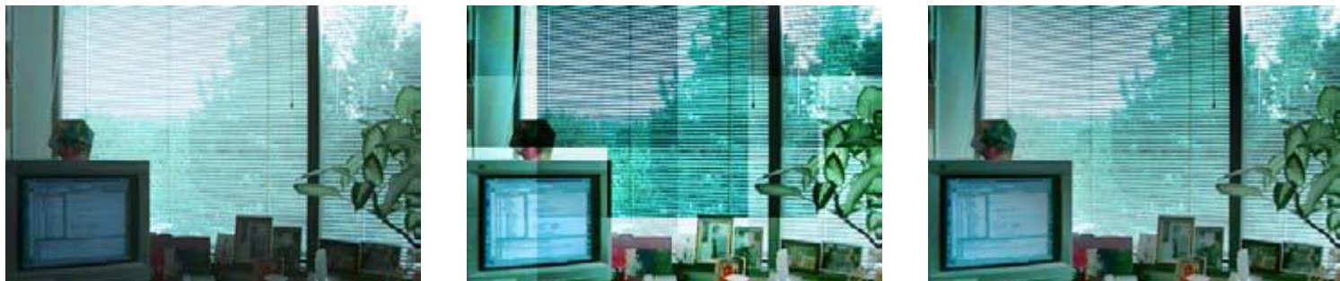
Figure 3.8 Locally adaptive histogram equalization: (a) original image; (b) block histogram equalization; (c) full locally adaptive equalization.
