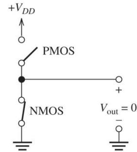
(c) Equivalent circuit with  $V_{in}$  high
