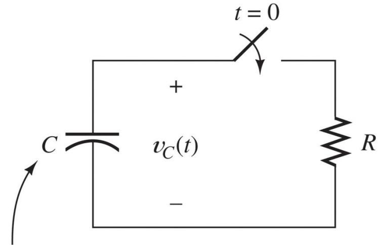
Capacitance charged to  $V_i$  prior to  $t = 0$
