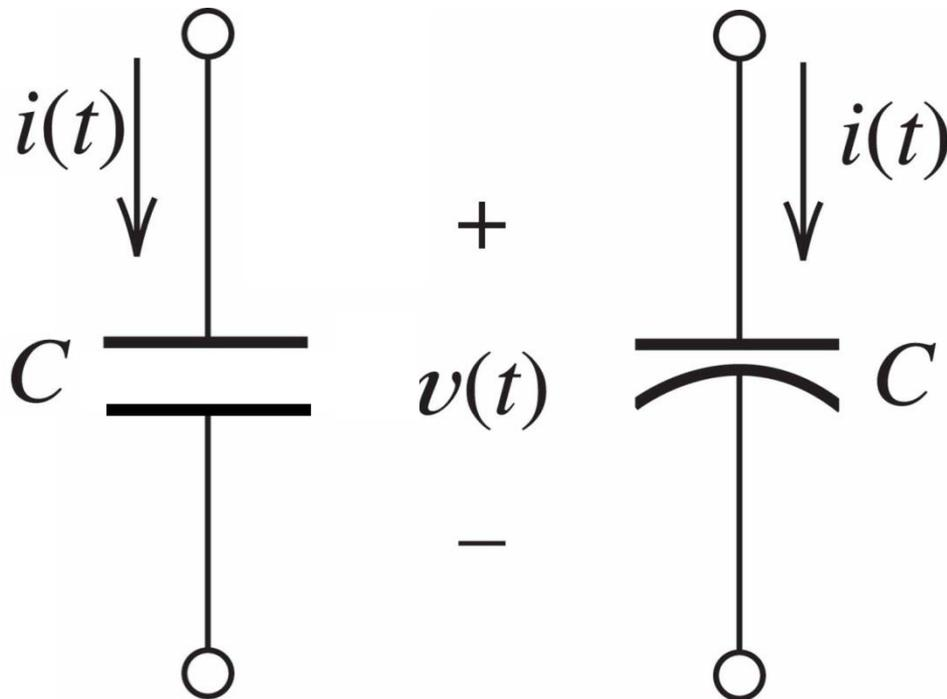
Curved capacitor is used for electrolytic capacitors which have explicit terminal polarity
