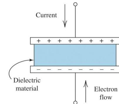
(a) As current flows through a capacitor, charges of opposite signs collect on the respective plates
