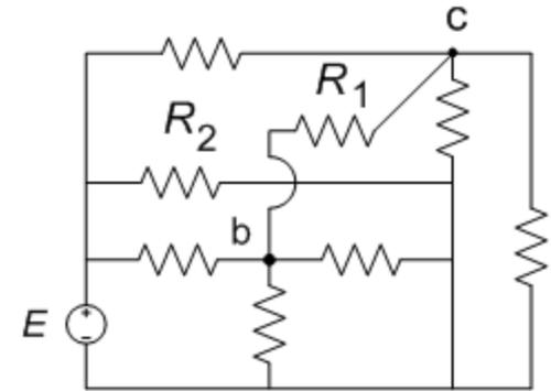
Fig. 5: A Non-Planar Circuit
