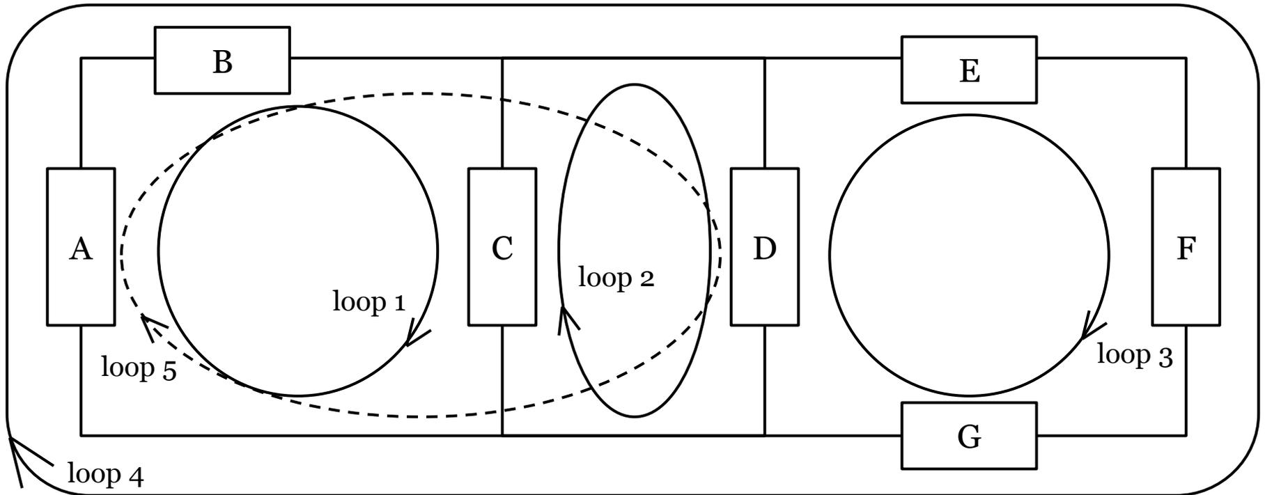
A loop is a closed path along circuit from a start node back to itself
