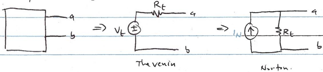
① open circuit voltage  $V_{OC} = V_T$
