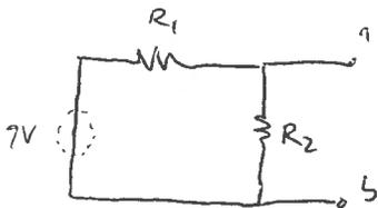
$$\begin{aligned} R_t &= R_1 \parallel R_2 \\ &= \frac{6 \cdot 12}{6 + 12} = \frac{72}{18} \\ &= 4\Omega \end{aligned}$$
