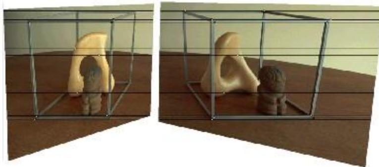
(c) Image pair transformed by the similarity H_r and H'_r . Note that the image pair is now rectified (the epipolar lines are horizontally aligned).
