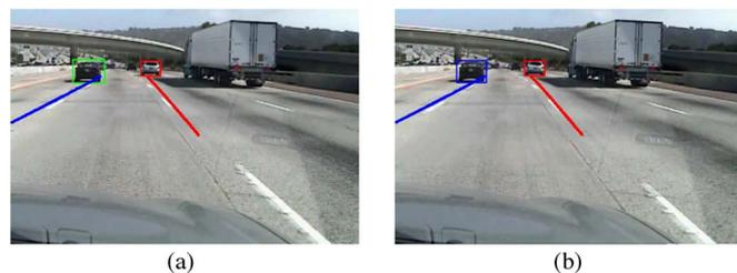
Fig. 15. Ambiguities in lane/vehicle positions. The vehicle on the left is in the midst of a lane change. (a) Vehicle is determined to still be in the ego-lane. (b) Vehicle is determined to have changed lanes in to the left lane. (a) Frame 519. (b) Frame 520.
