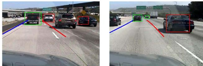
Fig. 11. (a) Poor lane localization due to a missed vehicle detection. The missed vehicle detection leads the lane tracker to integrate erroneous lane markings into the measurements, resulting in worse lane estimation for the right marker. (b) Example misclassification of lane position. The jeep in the right lane (green) has been classified as in the ego-lane. This is due to the fact that the jeep is farther ahead than the lane tracker's look-ahead distance.
