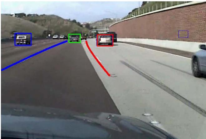
Fig. 2. Typical performance of integrated lane and vehicle tracking on highway with dense traffic. Tracked vehicles in the ego-lane are marked green. To the left of the ego-lane, tracked vehicles are marked blue. To the right of the ego-lane, tracked vehicles are marked red. Note the curvature estimation.
