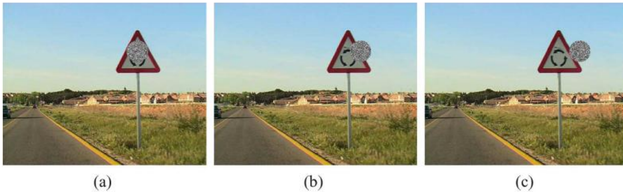
Fig. 26. Masks of occlusion. Three sizes are used to test the robustness of the system against occlusions with different areas covered. (a)–(c) Masks whose diameters are one half, one third, and one fourth of the major dimension of the bounding box, respectively.
