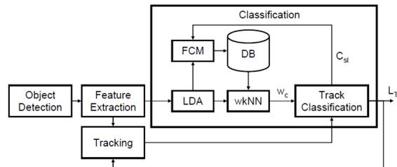
Fig. 8. Block diagram for the VECTOR classification scheme.
