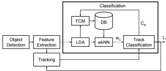
Fig. 3. Block diagram for the proposed classification scheme.
