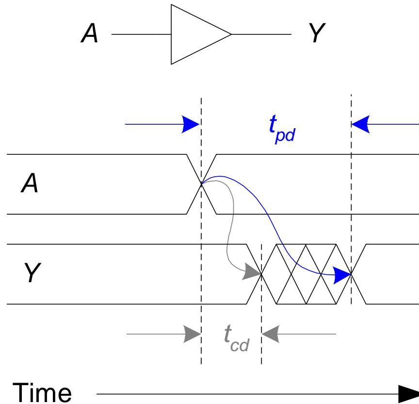
Note: Timing diagram shows a signal with a high and low and transition time as an 'X'.
