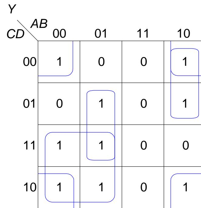
$$Y = \bar{A}C + \bar{A}BD + \bar{A}BC + \bar{B}\bar{D}$$
