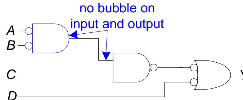
$$Y = \overline{A}\overline{B}C + \overline{D}$$
