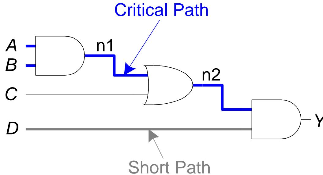
**Critical (Long) Path:**  $t_{pd} = 2t_{pd\_AND} + t_{pd\_OR}$
