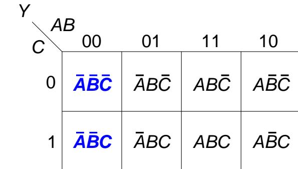
$$Y = \bar{A}\bar{B}\bar{C} + \bar{A}\bar{B}C = \bar{A}\bar{B}(C + \bar{C})$$
