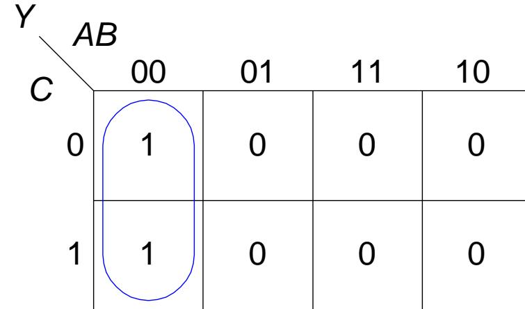
$$Y = \bar{A}\bar{B} \quad C \text{ not included because both } C \text{ and } \bar{C} \text{ included in circle}$$
