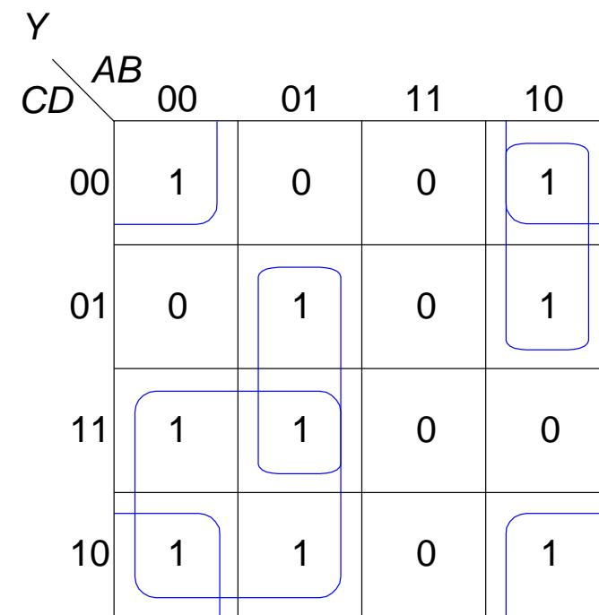
$$Y = \bar{A}C + \bar{A}BD + A\bar{B}\bar{C} + \bar{B}\bar{D}$$
