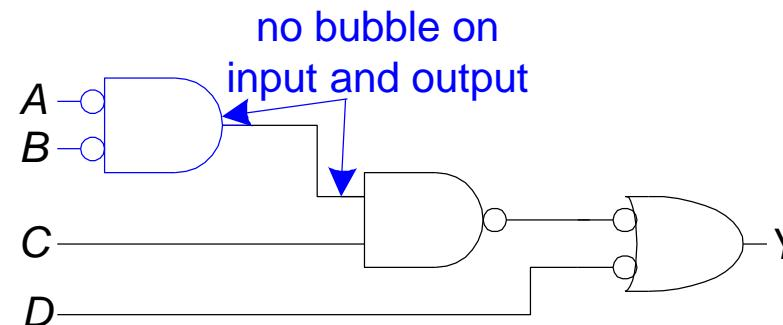
$$Y = \overline{A}\overline{B}C + \overline{D}$$
