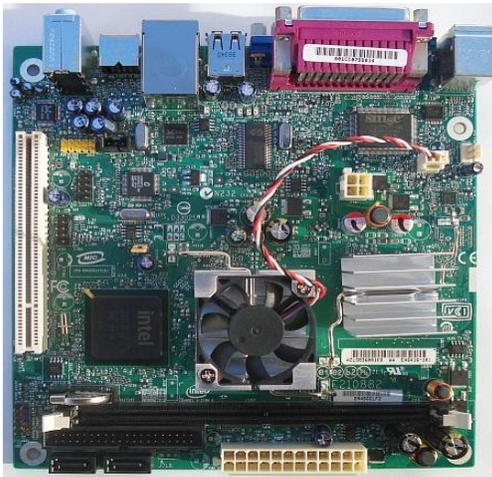
Figure 1. Intel Atom motherboard includes a fan for heat dissipation [8]
