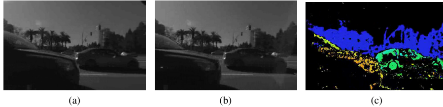
Fig. 5: Side looking stereo camera configuration for blind spot monitoring.
