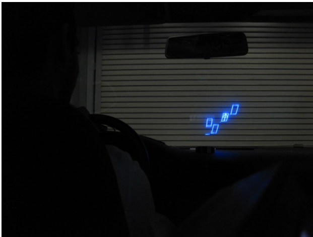
Fig. 8: Heads up display with prototype surround vehicle display. The dynamic active display (DAD) is a laser-based wide-area heads-up windshield human interface system.
