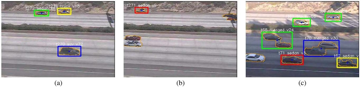
Fig. 6. User-defined speed profiling. (a) Car slowing (yellow box) before stopping on the shoulder. (b) Car coming to rest (red box) on the shoulder of the highway. (c) Friday evening high volume traffic showing merging of vehicles. The north- and southbound directions have different speed profiles because of southbound congestion.
